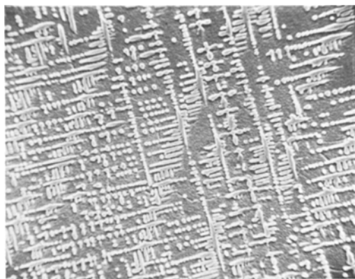
Figure 5 Microstructure of a 20 wt% Nb-Cu alloy chill cast from a Y 2 O 3 crucible under conditions identical to Fig. 3 (× 700).
